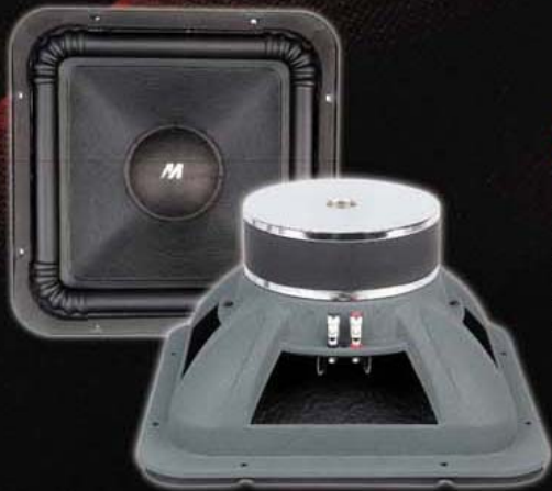
Stamped Basket Paper Cone With Rubber Edge
