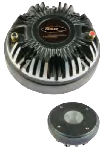
PRO-D002 High Frequency Driver Titanium Diaphragm 2" CCAW Voice Coil 33oz Ferrite Magnet Impedance: 4 / 8 Ohm Power: 400WRMS / 800WMAX Frequency Response: 2KHz-20KHz Sensitivity: 105dB 1W/1M
