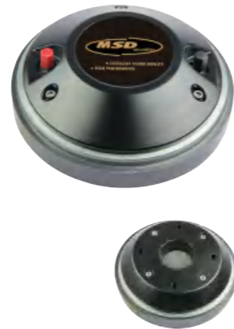
PRO-D003 High Frequency Driver Titanium Diaphragm 3" CCAW Voice Coil 68.2oz Ferrite Magnet Impedance: 4 / 8 Ohm Power: 500WRMS / 1000WMAX Frequency Response: 2.5KHz-20KHz Sensitivity: 107.5dB 1W/1M
